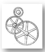
Centre lathes, like the ones found in school workshops, have compound gear trains that transmit rotary motion from an electric motor through to the headstock spindle. The leadscrew, which allows the tool post to travel on automatic feed, also operates from this compound gear train. Compound gear trains involve several pairs of meshing gears. They are used where large speed changes are required or to get different outputs moving at different speeds.
